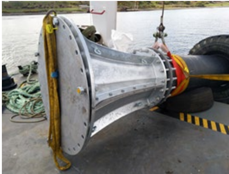
Plate 4-13: Example of bellmouth used to protect the duct ends at the HDD exit point (Source: Equinor)
